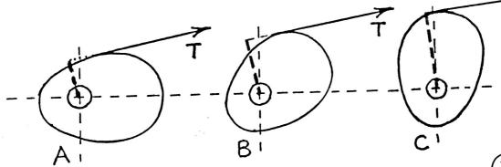
a. Draw the different-length lever arms for positions B and C. (Take care that your lever arm is perpendicular to the line of action of T!) The cam provides a changing lever arm!
