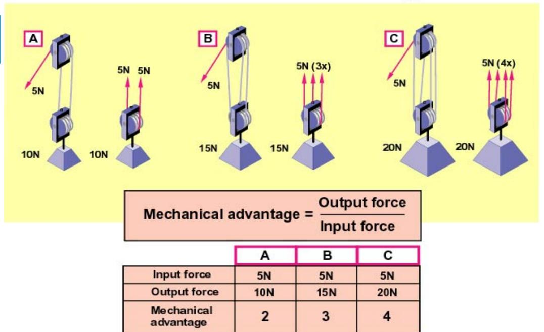
**PULLEYS** Like levers and ramps, pulleys sacrifice displacement for greater forces: pull greater displacement = apply less forces MA is shown by how many ropes are supporting the "load"
