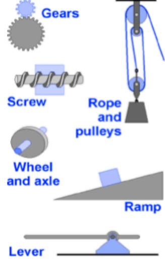
MACHINES Think about machine in terms of **input** and output Still constrained by conservation of energy At absolute best:  $W_{in} = W_{out}$  $(_{F}d)_{in} = (F_{d})_{out}$
