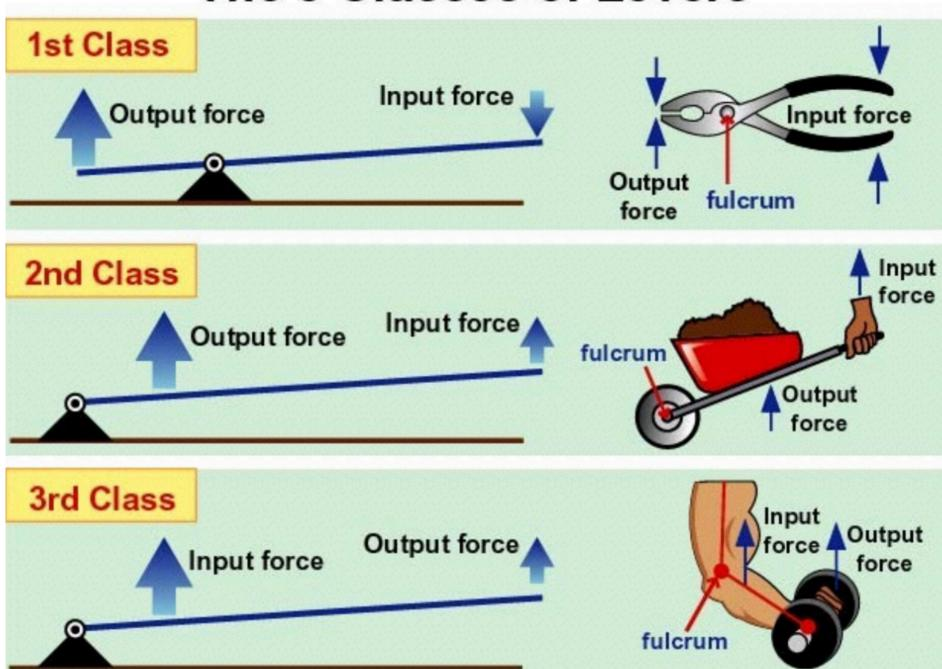
LEVER MECHANICAL ADVANTAGE (MA)  $MA_{lever} = L_{in}/L_{out} (=F_{out}/F_{in})$ What force must be applied to the end of a 2.0 m long crowbar in order to lift a 500N rock if the fulcrum of the bar is 0.5 m from the rock?
